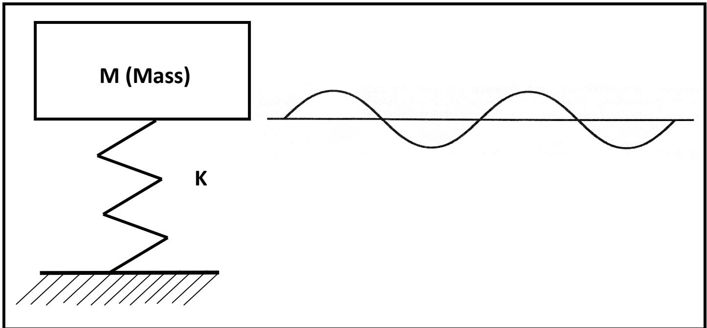
**Figure 1.** Schematic of a single degree of freedom dynamic system where the mass,  $M$ , is the vibratory source.
