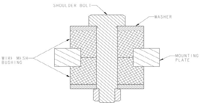
**Figure 13.** Isolator with wire mesh load carrying pad.
