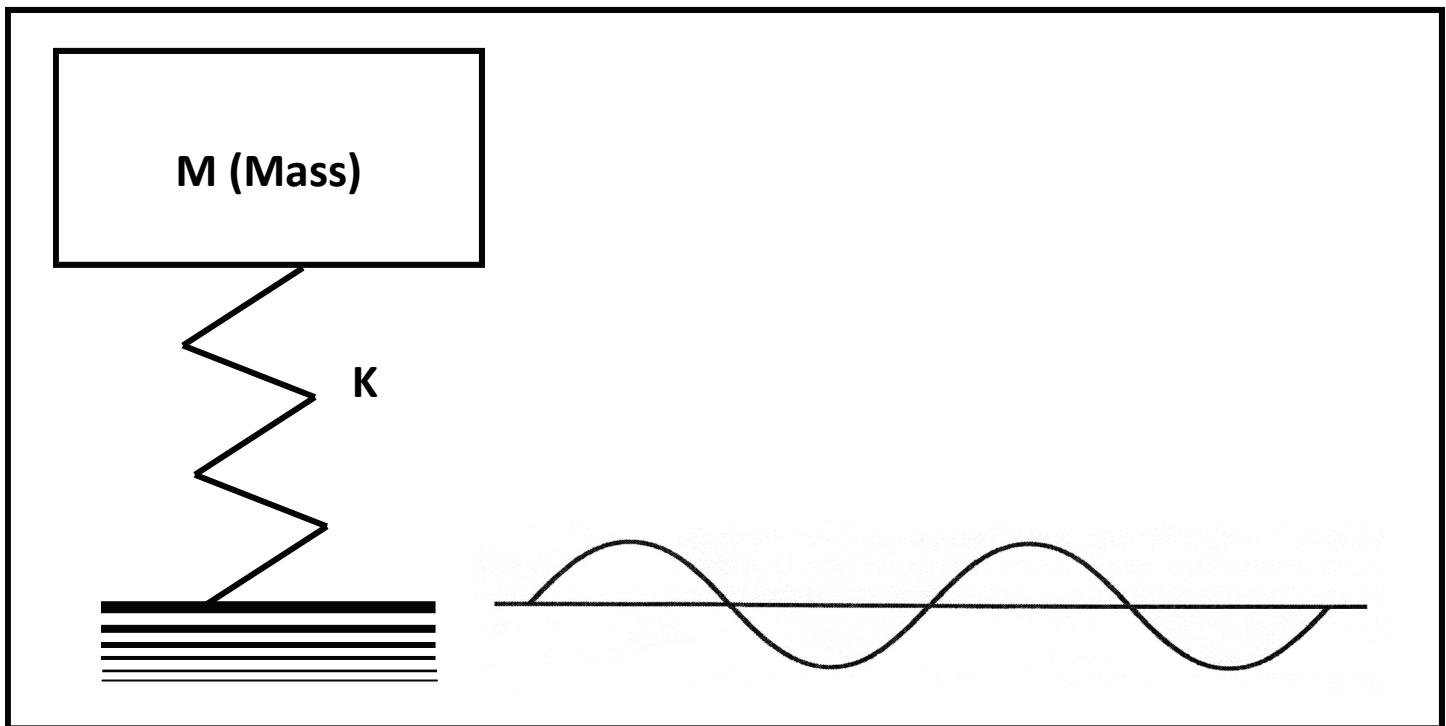
**Figure 2.** Schematic of a single degree of freedom dynamic system where the floor is the vibratory source.
