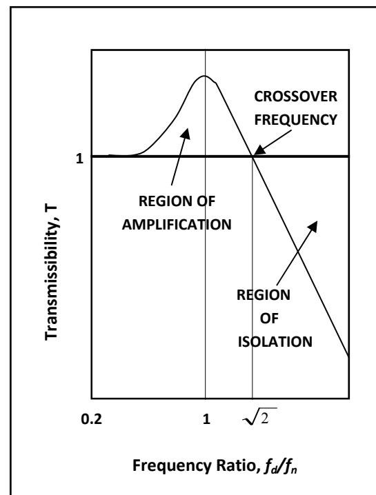
**Figure 6.** Transmissibility curve for an isolated system where  $f_d$  = disturbance frequency and  $f_n$  = system natural frequency.
